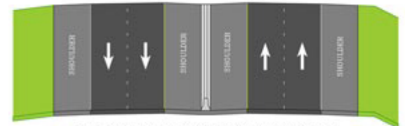
PROPOSED I-75 MAINLINE W/ MEDIAN BARRIER APPROXIMATE LIMITS: 4TH STREET TO SR 81
